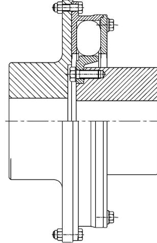
Shaft to Shaft Coupling. Designed for use on electric motor drives and power take off applications.
