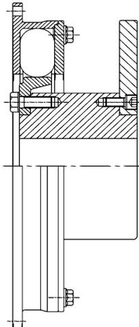
Coupling with additional inertia on the inner mass
