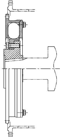
Existing hub fitment. Coupling inner member designed to suit existing hub design.
