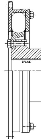
Coupling with limited end float for splined input shafts
