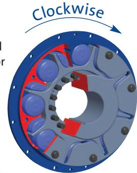
It is important, therefore, to establish which direction the coupling will operate at the specification stage. The coupling shown here is designed to operate in a clockwise direction.
