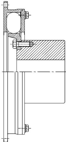
Coupling with reversed inner member to increase distance between flywheel face and shaft end.
