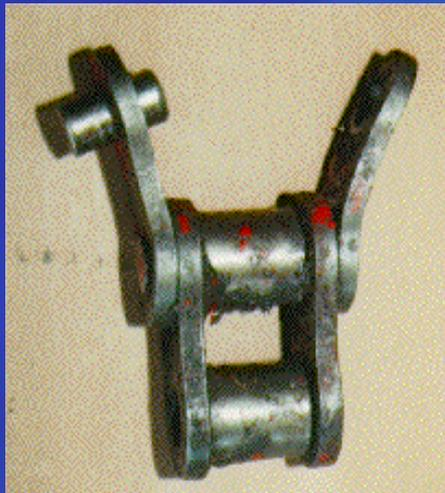
Overload failure can also cause the pin to break
